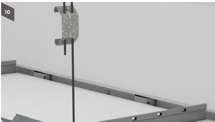
10 Secure all perimeter tiles with U-Trim using butterfly clips, which will function as springs to push the tiles towards the grid.
