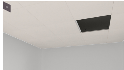
8 Install the S-BESK tile. Individually demount each tile in this system for maintenance. To remove any tile, slightly raise the tiles on one side until they can be slid off the main profile.
