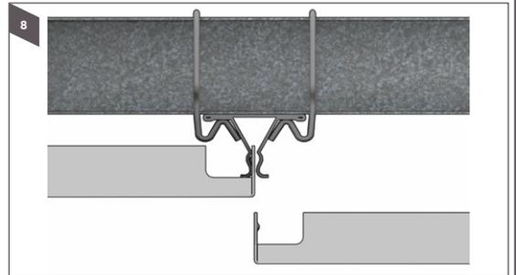
Insert the clip in panel to the exposed spring tee
