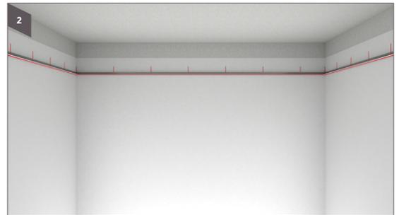
2 Install wall angles around the perimeter at marked locations using screws at 450 mm o.c
