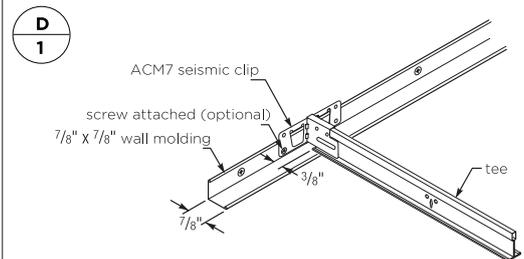
All main DONN® suspension systems - DX/DXL, Finline DXF, Finline 1/8 DXFF, Centricitee DXT/DXLT, CE, DXW, DXLA, and ZXLA - include the Code compliant intermediate-duty main tees for Seismic Design Categories A, B and C.
