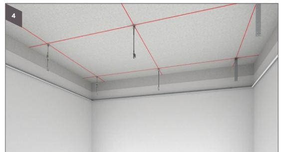
4 Fix hangers at 1200 mm o.c in a gradient scheme above the lines of wall angle
