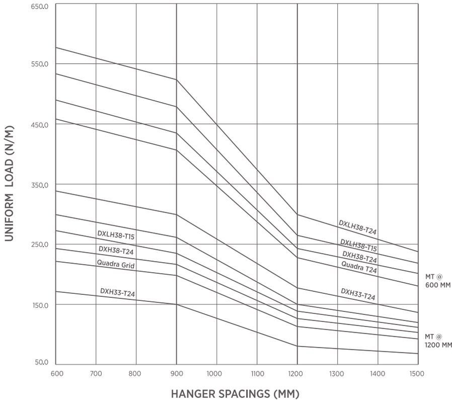
Minimum load carrying capabilities of main runners spaced at 1200mm and 600mm On Center.
