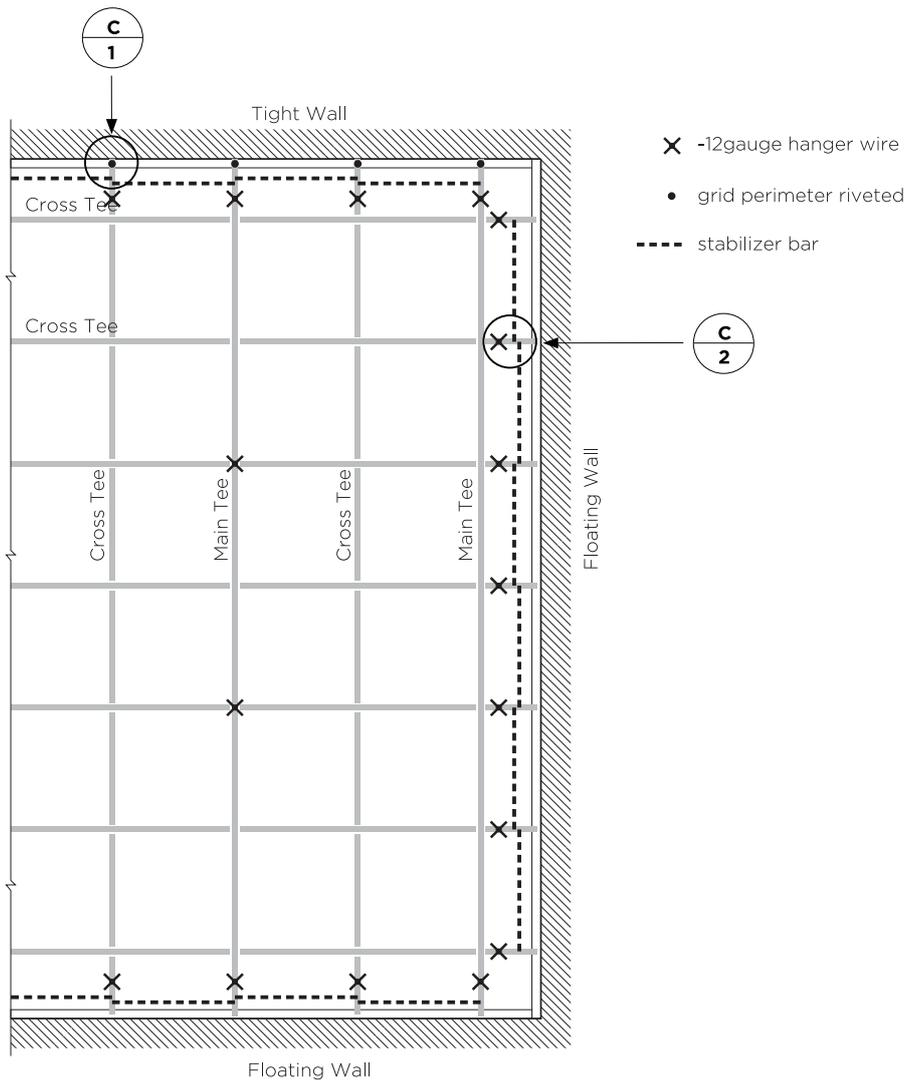
All main DONN® suspension systems – DX/DXL, Finline DXF, Finline 1/8 DXFF, Centricitee DXT/DXLT, CE, DXW, DXLA, and ZXLA – include the Code compliant heavy-duty main tees for Seismic Design Categories D, E, and F.
