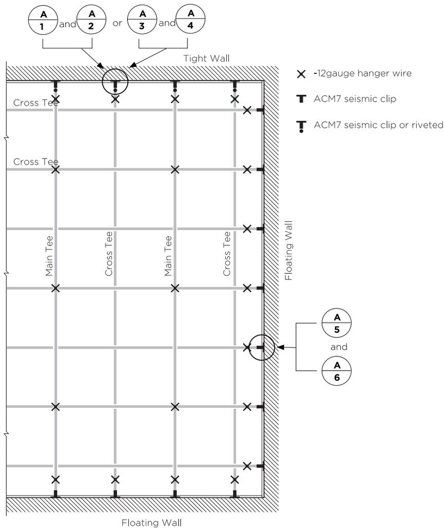
All main DONN® suspension systems - DX/DXL, Finline DXF, Finline 1/8 DXFF, Centricitee DXT/DXLT, CE, DXW, DXLA, and ZXLA - include the Code compliant and heavy-duty main tees for Seismic Design Categories D, E, and F.
