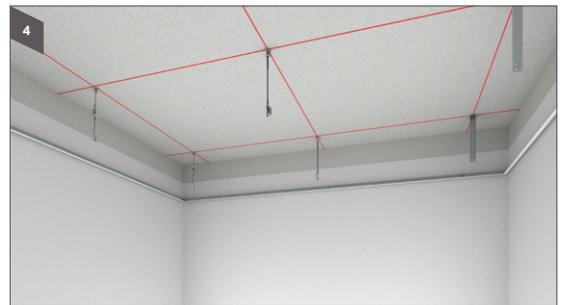
4 Fix hangers at 1200 mm o.c in a gradient scheme above the lines of primary channels
