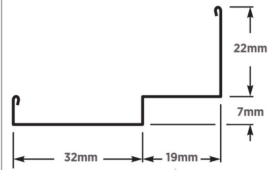
Preformed corners are available, eliminating the need to miter this molding.
