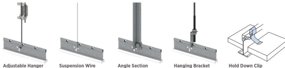
Adjustable Hanger      Suspension Wire      Angle Section      Hanging Bracket      Hold Down Clip
