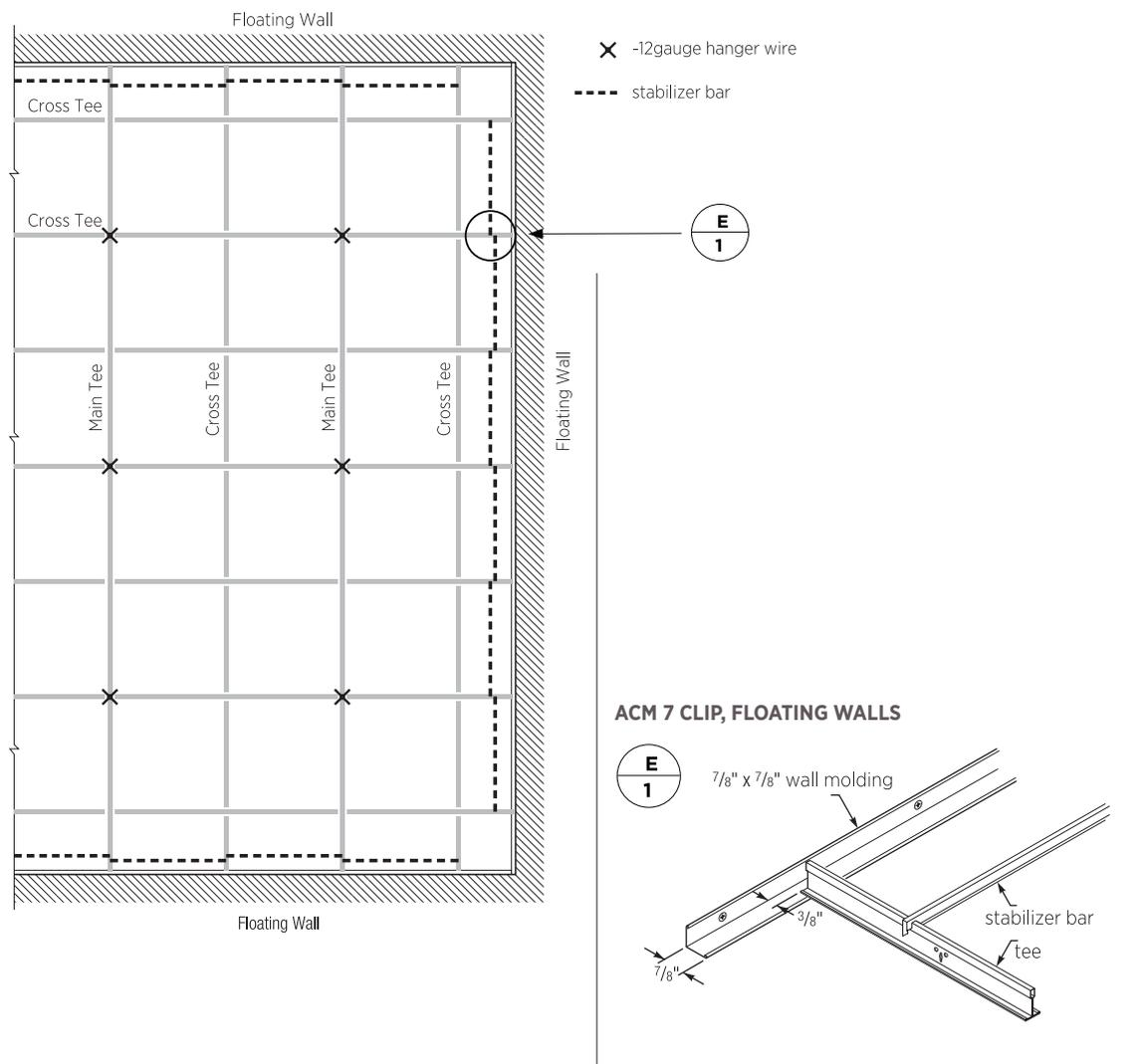
All main DONN® suspension systems – DX/DXL, Finline DXF, Finline 1/8 DXFF, Centricitee DXT/DXLT, CE, DXW, DXLA, and ZXLA – include the Code compliant intermediate-duty main tees for Seismic Design Categories A, B and C.
