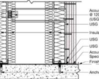
Acoustical Bracing Installed @ 1200mm(min), 1800mm(max) (USG Acoustic V-Brace) USG Stud as per Design (G90)
