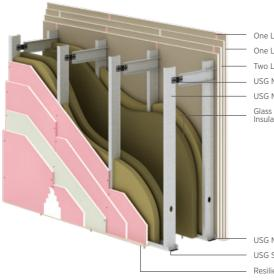
One Layer USG Sheetrock® Type X 15.9 mm One Layer Sheetrock® Regular 12.7 mm Lavers USG Sheetrock® Type X 15.9 mm JSG ME Acoustic V Brace USG ME C Stud 90.5\*0.9 mm Glass Wool Insulation and Stone Wool
