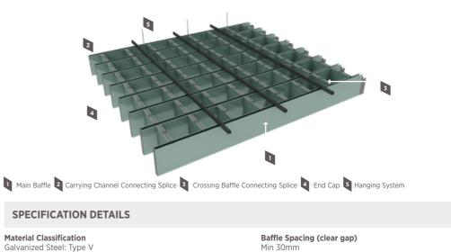
Light Reflectance Coefficient [LR] Based on the finish color and perforation pattern, LR up to 0.82 Surface Burning Characteristics per ASTM E 84 Class A Color Standard colors are RAL 9016, RAL9006 and RAL9010. Other RAL colors are available upon request Additional Information • Recommended spacing is to be equal to the height of the baffle Thickness depends on panel sizes and project requirements
