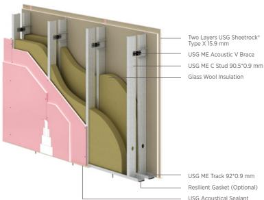
USG ME Track 92\*0.9 mm Resilient Gasket (Optional) USG Acoustical Sealant
