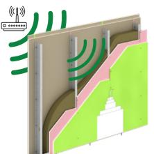
The construct of a third-party laboratory tested STC 55 partition made from AAC block versus drywall system.
