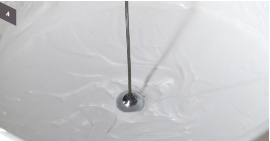
Step 4 Check the viscosity of the paint using the material thickness gauge (small steel ball)
