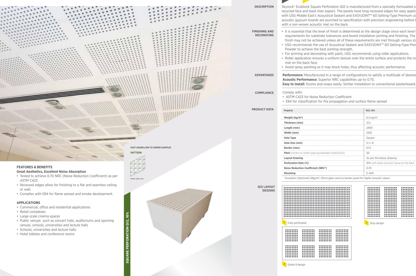
Skyrock® Ecoblock Square Perforation Q12 is manufactured from a specially formulated core encased in recycled face and back liner papers. The panels have long recessed edges for easy application when used with USG Middle East's Acoustical Sealant and EASYJOINT™ 60 Setting-Type Premium-Jointing Powder. The acoustic gypsum boards are punched to specification with precision engineering before being laminated
