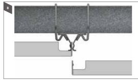
Connect the spring tee to the primary channel at 600 spacing Insert the clip in panel to the exposed spring tee using wire connecting clip WCC
