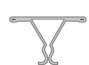
Spring T Channels are concealed and attached to main primary channels through wire connecting clips.
