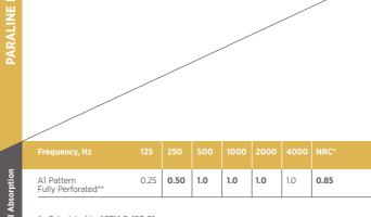
\* Calculated to ASTM C 423-01 \*\* Acoustic Fleece and 38mm Soft Fiber Infill
