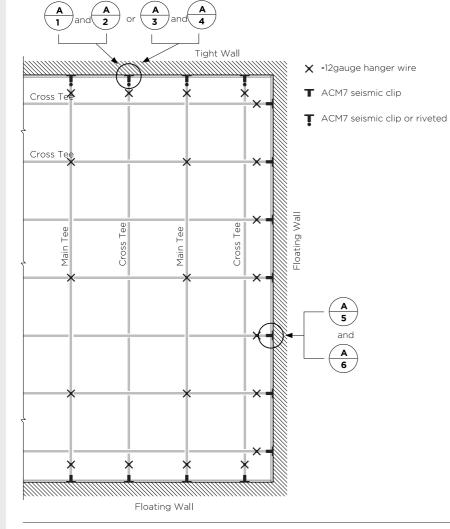
All main DONN<sup>®</sup> suspension systems – DX/DXL, Fineline DXF, Fineline 1/8 DXFF, Centricitee DXT/DXLT, CE, DXW, DXLA, and ZXLA – include the Code compliment and heavy-duty main tees for Seismic Design Categories D, E, and F.
