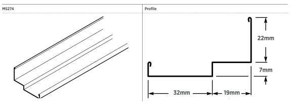
Preformed corners are available, eliminating the need to miter this molding.
