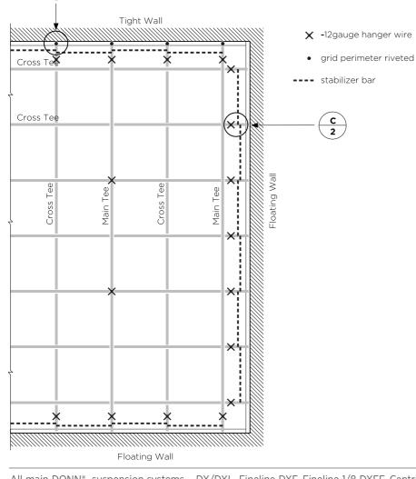
All main DONN<sup>®</sup> suspension systems – DX/DXL, Fineline DXF, Fineline 1/8 DXFF, Centricitee DXT/DXLT, CE, DXW, DXLA, and ZXLA - include the Code compliment heavy-duty main tees for Seismic Design Categories D, E, and F.
