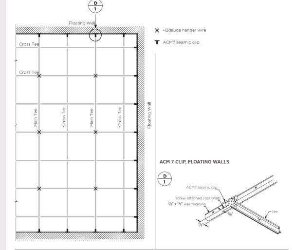
All main DONN<sup>®</sup> suspension systems - DX/DXL, Fineline DXF, Fineline 1/8 DXFF, Centricitee DXT/DXLT, CE, DXW, DXLA, and ZXLA - include the Code compliment intermediate-duty main tees for Seismic Design Categories A, B and C.
