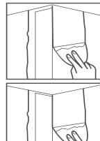
3. For inside corners apply compound to one side, let dry, then apply compound another coat of compound, feathering beyond prior coat, let dry. If needed smooth with wet sponge. Sand the surface after compound dries, sand with a wet sponge to eliminate dust or use 150-grit or finer sandpaper or 220-grit or finer abrasive mesh cloth. Avoid scuffing panel paper.
