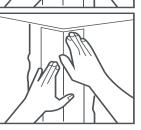
2. Fold tape at center. With the metal side of tape facing drywall surface, embed tape firmly to the other side. Apply in compound. Remove extra compound with taping knife. Allow to dry.
