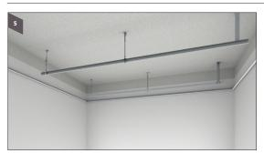
Fix the primary channel at 1200 mm spacing
