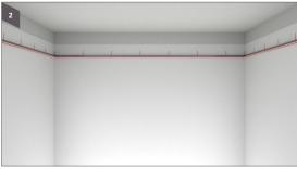
Install wall angles around the perimeter at marked locations using screws at 450 mm o.c
