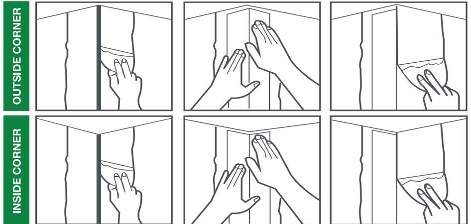
1. Apply over dry surface only. Maintain minimum air, joint compound and surface temperature of 15°C until joint compound is completely dry. Using a 150 mm knife, apply joint compound to inside or outside corner of drywall.
