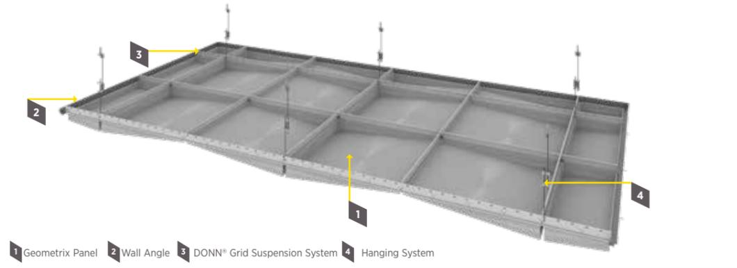
1 Geometrix Panel 2 Wall Angle 3 DONN® Grid Suspension System 4 Hanging System
