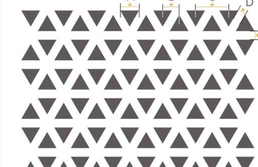
Triangular Pattern. Triangle Size (A): 10mm, Pitch (B): 9.16mm, Pitch (C): 18.32mm, (D): 4.8mm, Open Area: 30%
