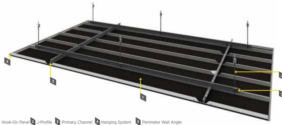
1 Hook-On Panel 2 J-Profile 3 Primary Channel 4 Hanging System 5 Perimeter Wall Angle
